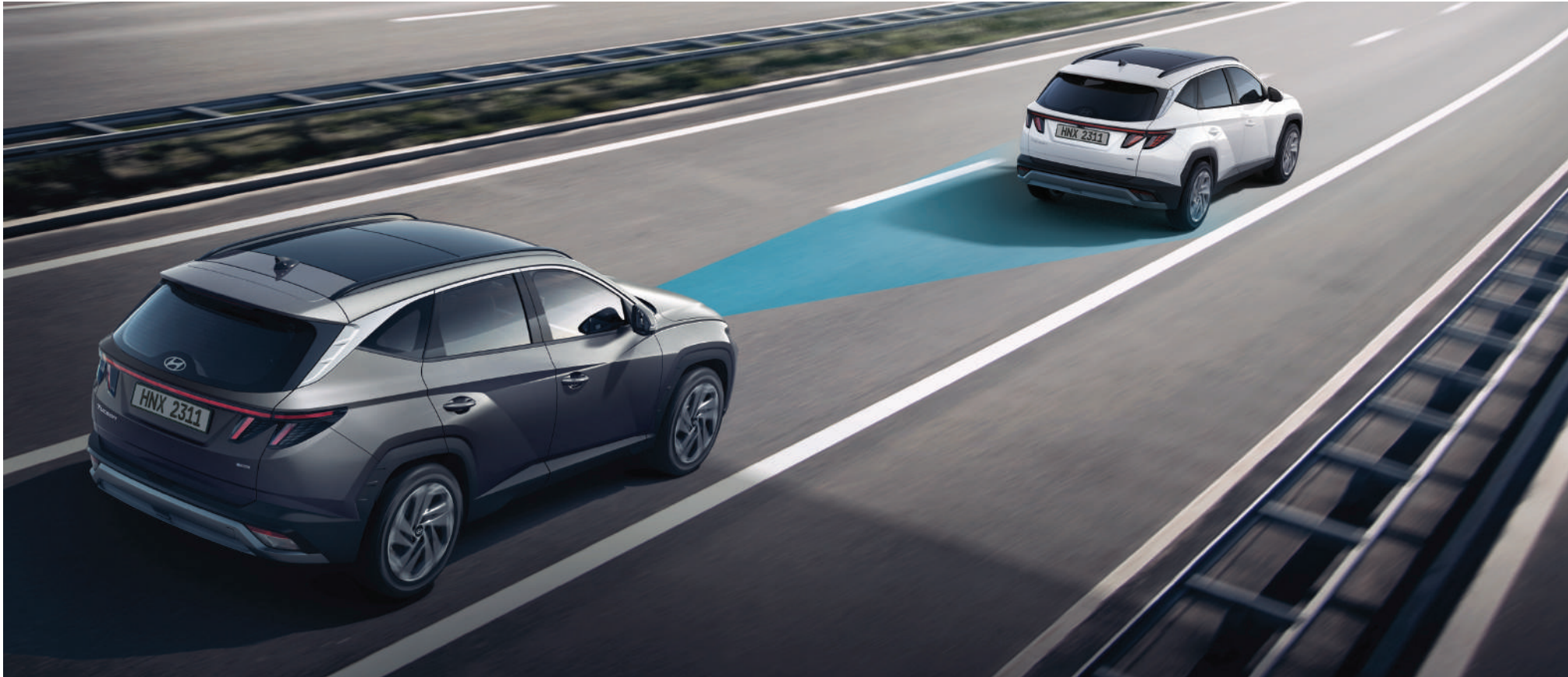
Smart Cruise Control (SCC) with Stop and Go Smart Cruise Control (SCC) helps maintain distance from the front vehicle and drive at a speed set by the driver. Automatically stops when the front vehicle stops and automatically starts when the front vehicle departs within a short time.
